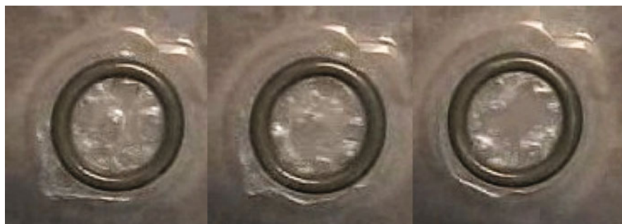
Fig. 12.14 Traveling and decaying of cnoidal waves on the external contour taken at three different moments of time
